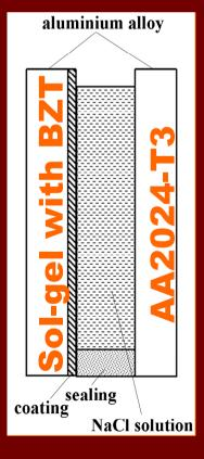
Cells were filled with 35 g l<sup>-1</sup> NaCl solution for (a) 5 h and (b) 200 h.
